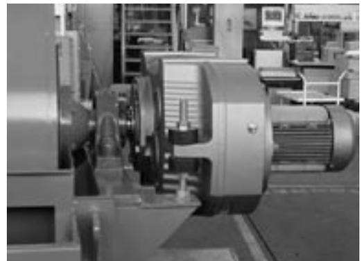
Direct Drive - Shaft Mounted Gearmotor
