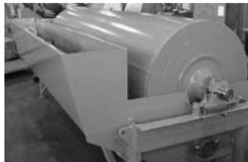
All Stainless Steel Tank and Feedbox Construction
